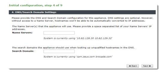
The Traffic Manager works correctly without access to external name servers, however you then have to use IP addresses instead of hostnames when setting up pools of servers, or manually enter the hostname to IP mappings, which can be done from the Admin UI (in the "DNS" section of the **System > Networking** page) once you have completed the initial configuration wizard.
