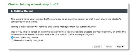
To instruct the Traffic Manager to automatically scan the network for contactable Traffic Managers, click "Select existing cluster". Alternatively, to enter a specific hostname and port you want to join, click "Manually specify host/port".
