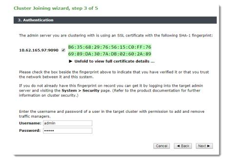
Check the displayed SHA-1 fingerprint against the fingerprint shown in the target Traffic Manager's Admin UI, in **System > Security**.
