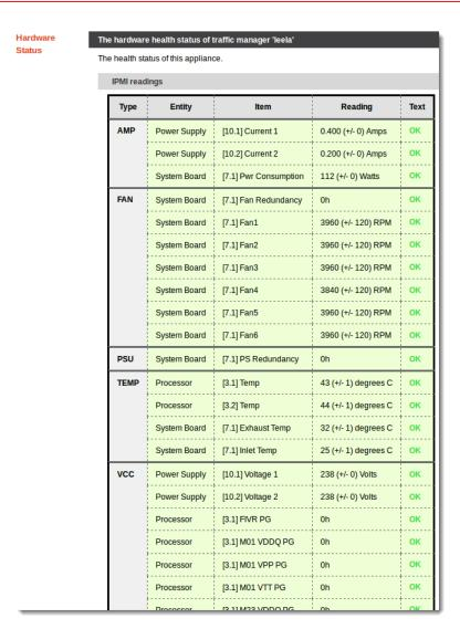
The Hardware Status page provides a list of hardware devices present in the appliance. Each device section contains a list of parameters along with the current reading and overall health state of that parameter.
