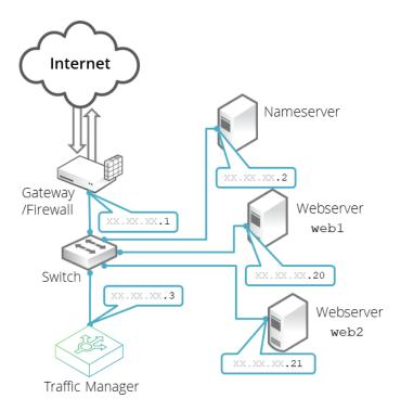
By installing a Traffic Manager, configured to receive traffic over a single network port and IP address xx.xx.xx.3, you can alter your DNS record to instead direct clients to xx.xx.xx.3. In this way, the Traffic Manager receives the Web page requests and responds with content from one of the available Web servers.
