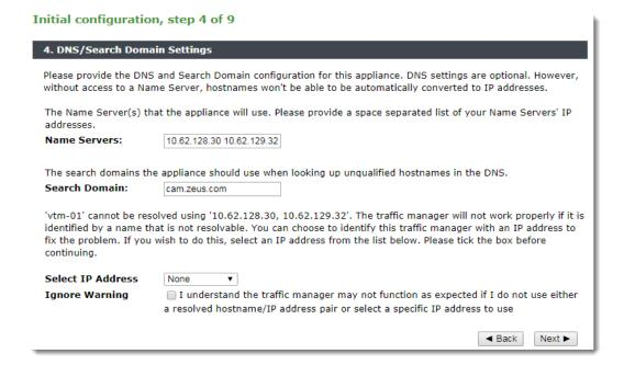
Select the desired IP address from the drop-down list, or select "None" to force the wizard to set the Traffic Manager name to be the unresolvable hostname. However, you can experience connectivity issues until the hostname successfully resolves to an IP address within your DNS. Read and confirm your acknowledgement of the Ignore Warning message by clicking the checkbox provided.
